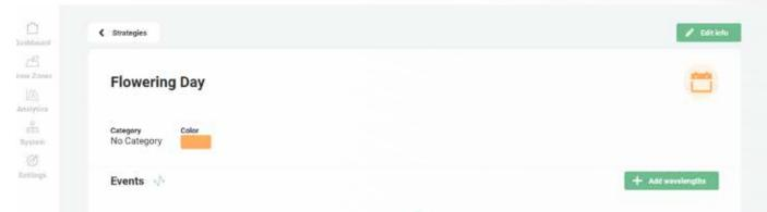
An event is each instance of changing light intensity or quality, as well as switching off the lights. Light intensity of separate wavelength/LED channels is programed by choosing numbers from 0 to 1000 which represent permilles ( $\infty$ ) of total current used by this LED channel. Between 200 and 900 it is fairy linearly related to light intensity.
