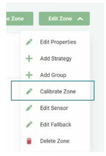
**To re-calibrate go to the Grow Zone page and choose Edit Zone.** This will show you the graph again, above the graph you will see a re-calibrate button. Click that and the lights and sensors will re-calibrate. When recalibrating you will see the lights switch off then come on at 100 then switch off and come back on at 1000. Once they have stopped blinking you can re-check the graph and you should have a curve closer to the one in this example.
