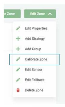
**To re-calibrate go to the Grow Zone page and choose Edit Zone.** This will show you the graph again, above the graph you will see a re-calibrate button. Click that and the lights and sensors will re-calibrate. When recalibrating you will see the lights switch off then come on at 100 then switch off and come back on at 1000. Once they have stopped blinking you can re-check the graph and you should have a curve closer to the one in this example.
