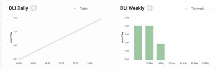
Four of the graphs are dedicated to the Smart Controllers and will only be visible if sensors are installed. The **DLI Daily** graph shows the accumulated light in the photo period for the date that you have selected. It is expressed in mol/m<sup>2</sup> over a 24 hour period. By hoovering over the graph you will be able to see the DLI value accumulated at that time of the day.
